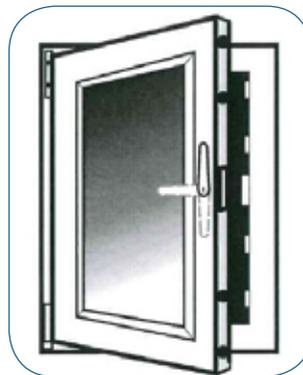
The term 'Tilt Before Turn' (TBT) refers to the sequence of operation of the window which is designed for safety, to initially select the 'Tilt' mode, followed by the 'Turn' mode.
